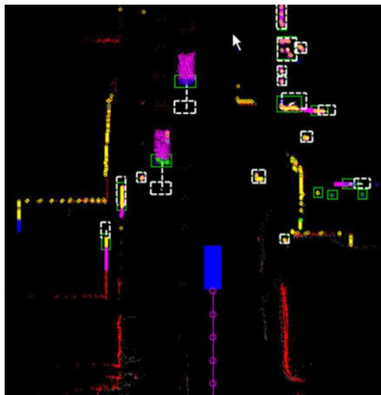
Figure 2.9. SLAM and DATMO with advanced algorithm [28]
